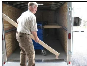
5. Unlock the wheel locks on the transporter cart. Roll the transporter cart off the trailer. A full transporter weighs approximately 315 pounds.
