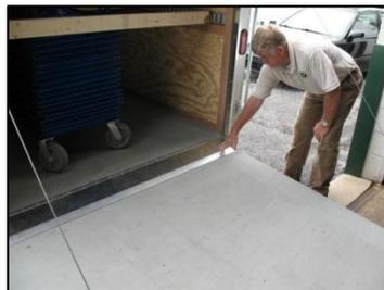
4. Remove the rear beam by pushing on the E-Track socket spring lever. Pull socket away from the E-Track while rotating downward until it is completely disengaged from the E-Track. Repeat for other side and remove the beam to a safe place.
